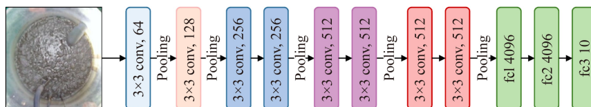
Fig. 2 Image feature extraction process.
